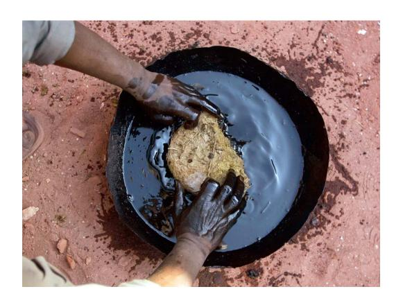
A worker soaks dry cow dung in a mixture of kerosene and gasoline at a kiln near Amritsar, India.
